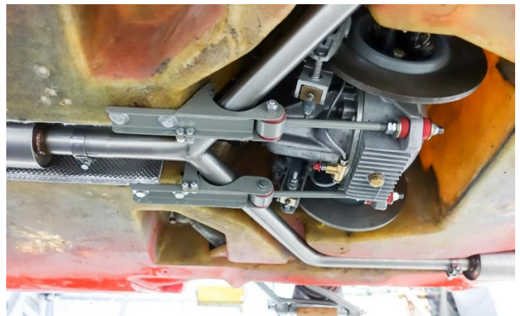
Figure 20 - Relocated lower stabilizing rods.
