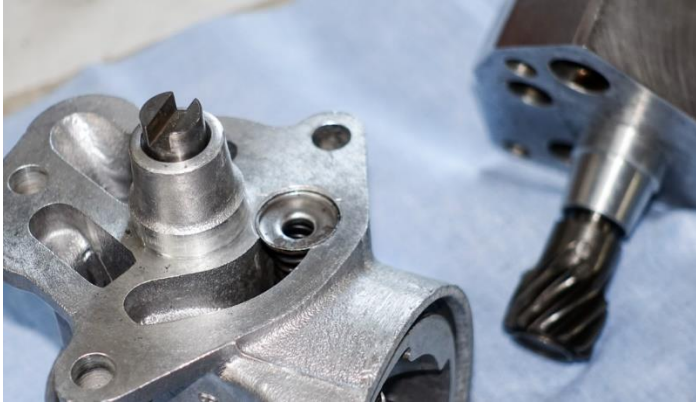
Figure 16 - Oil pump drive "slot"
