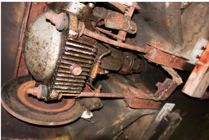
Figure 11 - The sub-frame/rubber mounted differential
