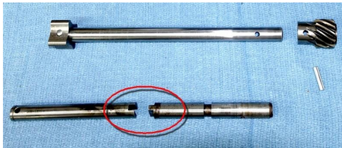
Figure 17 - Bifurcated shafts, and the replacement one-piece shaft
