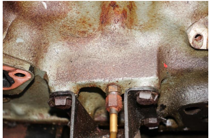
Figure 7 - This is where the serial number is normally located.
