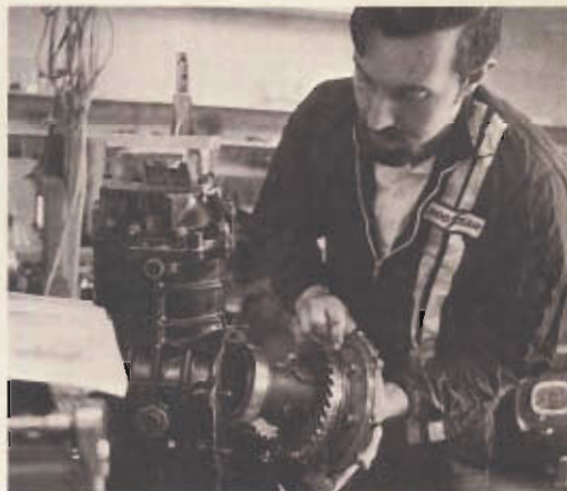
Right: A mechanic assembles a Volkswagen transmission and rear-end in the well-equipped Autodynamics workshop.
